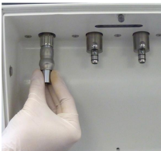
Figure 16: Change of turbine adaptor
