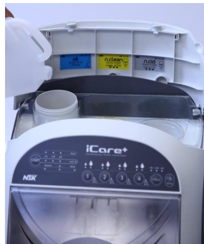
Figure 13: Filling the Oil tank of iCare+ device
