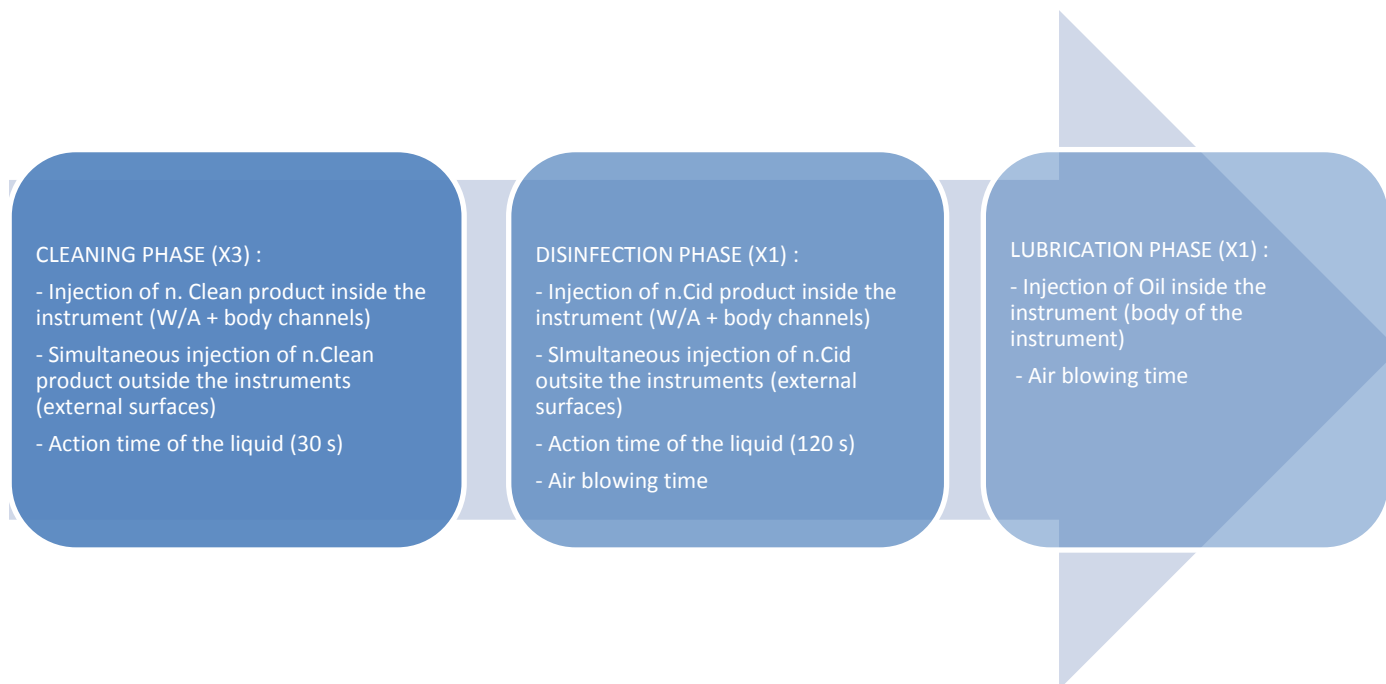
Figure 23: Treatment cycle of iCare+ device
