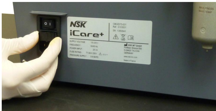
Figure 30: Fuse box of iCare+ device
