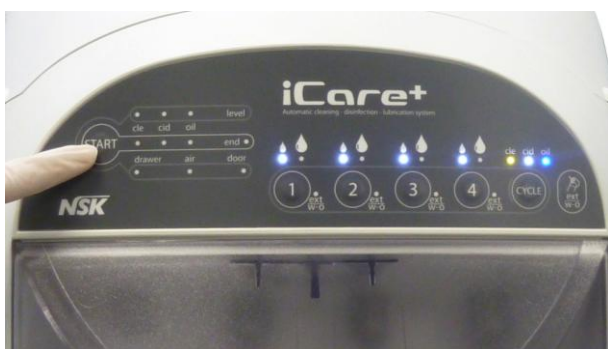
Figure 22: Launching the treatment cycle
