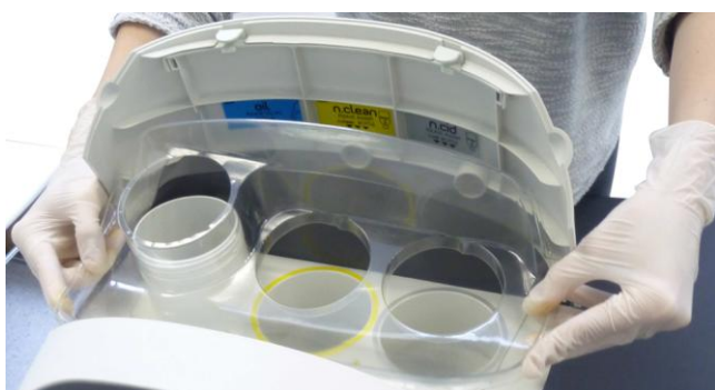
Figure 28: Replacement of the junction support blister
