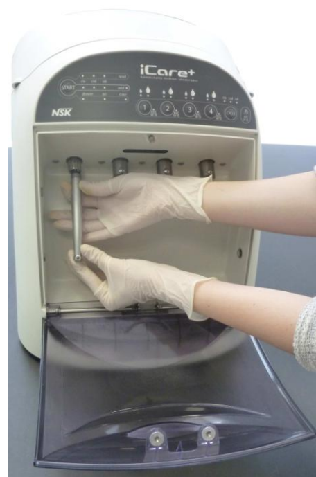
Figure 15: Screwing the ring on the Midwest coupling
