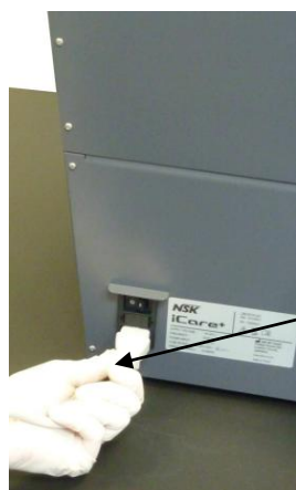
Figure 8: Electrical connection of iCare+ device
