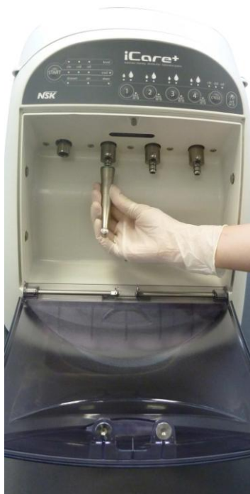
Figure 17: Connection of a contra-angle
