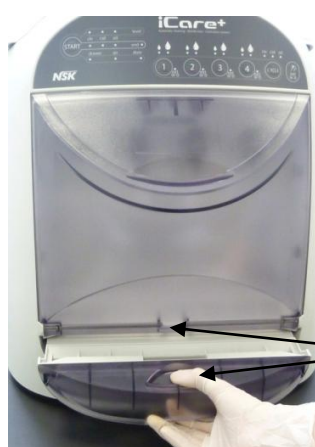
Figure 25: Removal of the drawer of iCare+ device
