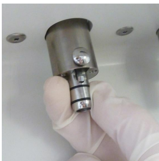
Figure 29: O-ring joints of E-type connector
