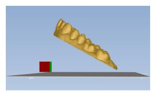
In these examples the models are lifted 3 mm and rotated to optimal positions so that anatomical surfaces are facing away from the build plate. In this position supports are not needed on any important surfaces.
