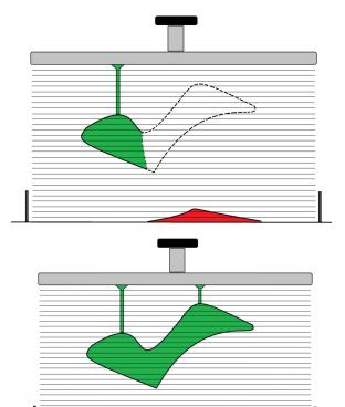
The most critical areas to support on a print model are the areas where initial contact is made relative to the build plate.
