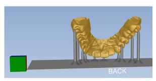
In this example the anatomical surfaces are compromised due to poor positioning and support placement.
