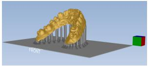
In this example the dental model is optimally supported and lifted 3mm from the build plate in a 45 degree angle.
