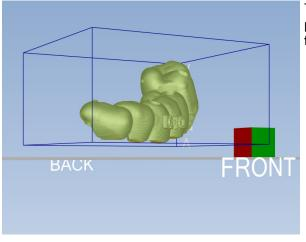
The imported model is positioned in contact with the build plate. To ensure more stable print lift the model 3-5mm from the build plate.
