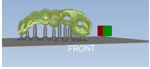
Here the guide model is supported in final optimal position.
