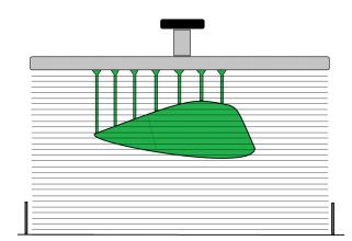
By adding supports also sloped surfaces can be printed successfully.
