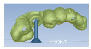
Here the model is positioned so that the geometrically sensitive sleeve hole has to be supported. This should be avoided to withhold the integrity of the sleeve hole geometry.
