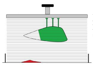
The need for additional supports increases when a print creates an angle less than 25 degrees to the build plate. If the slope is very low the part creates torsion and internal forces in the print. This significantly increases the possibility for failed prints.
