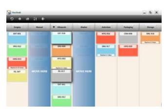
Using existing PCs or touch screen technology trays can be moved through the sterilisation process, noting where necessary, information about cycle parameters and success or failure of a cycle.
