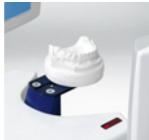
Scanning a plaster cast to a digital model
