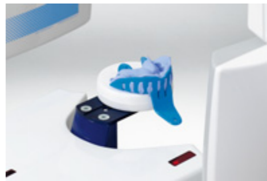
Scanning an impression to a digital model
