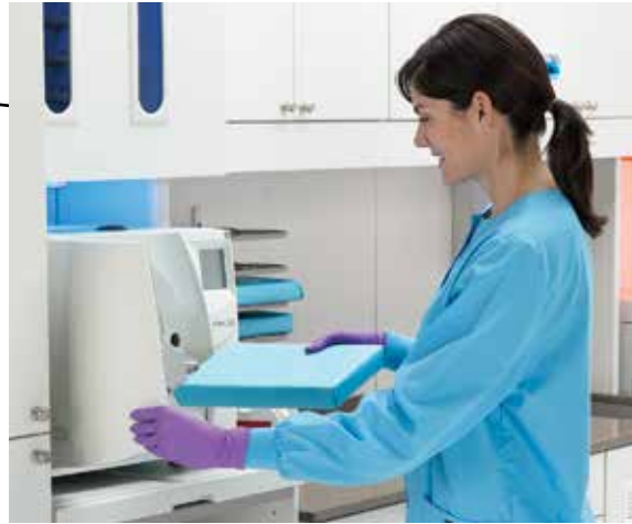
With a well-designed system, movement of items requires very little reaching or twisting. Here, the cassette is placed into the steriliser.
